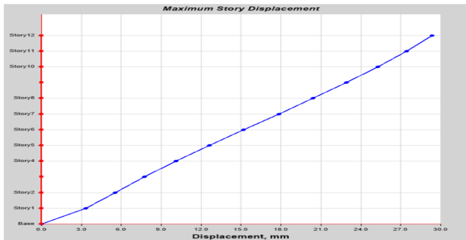
Fig. 11: Storey displacements in direction X at a storey of the structure without hanging columns
