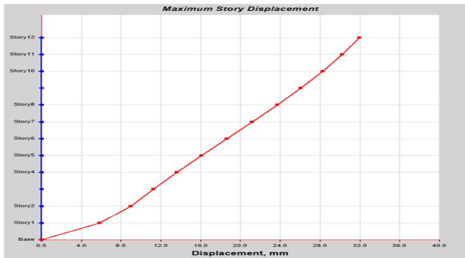
Fig. 12: Storey displacements in direction Y at a storey of the structure without hanging columns
